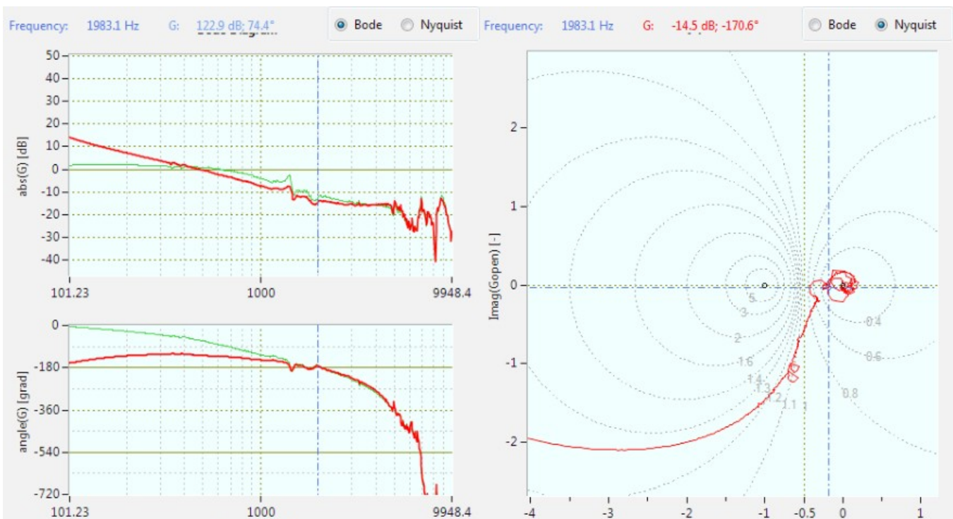
Figure 64: Notch2 filter with f_n = f_d = 2000\text{Hz} , D_n = 0.01 and D_d = 0.1 compensates the resonance.
